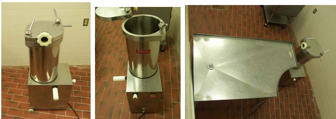
Figure 5. From left to right: front of automatic stuffer, profile of automatic stuffer, and automatic stuffer with its table.
