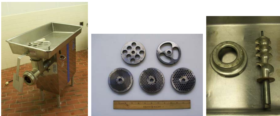
Figure 1. From left to right: meat grinder, grinding plates, and screw auger with cap.
