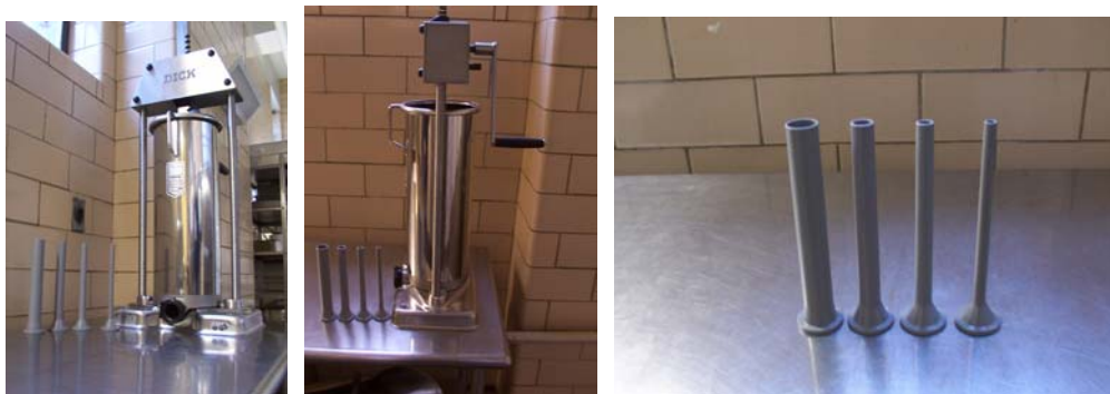
Figure 4. From left to right: front of hand crank stuffer, profile of hand crank stuffer, and stuffing horns.
